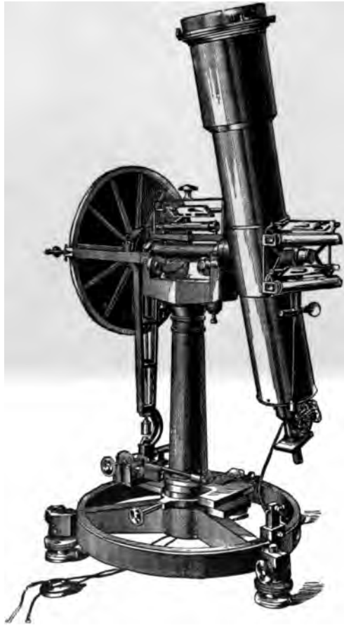
PHOTOGRAPHIC ZENITH TELESCOPE OF GEORGETOWN COLLEGE.
